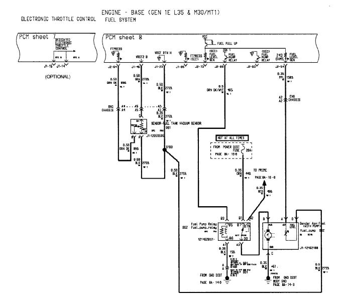
Figure 3.2.1a - XI - P/Truck - Mechanization Diagram - Fuel System and Optional ETC
